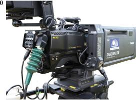
broadcast camera it is the green sensor that contains most of the image luminance. Using an extra green sensor, the SK-UHD4000 can deliver much higher resolution than three sensor 4K cameras at prices in the range of normal HDTV [2K] cameras.
